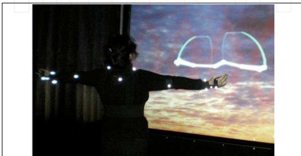
Fig. 9 .The gesture that represents “Sky” has been recognized. The user can see the avatar, hear the sound of a storm and see the picture of the firmament.
