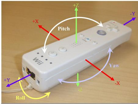
Fig. 2. Wiimote controller device with the reference axes.
