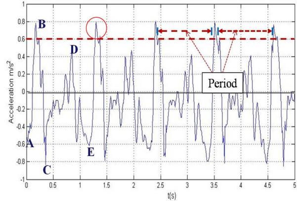
Fig. 3. Vertical acceleration of the walking gait over time.
