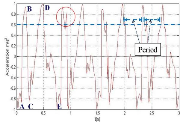
Fig. 4. Vertical acceleration of the running gait over time.
