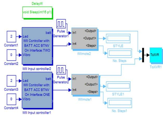
Fig. 10. Simulink model of the solution. The first output is the one that send the style to XVR, the second scope display the styles (1: stop, 2: walking, 3: run) and the last scope display the number of steps of the user during interaction.
