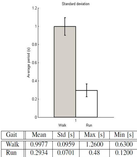
Fig. 8. Mean and standard deviation of the period between acceleration peaks (walking and running gaits).
