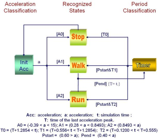
Fig. 9. State flow algorithm of the main solution, Pstart represents the beginning of acceleration peak and Pend represents the end of the acceleration peak see figures 3 and 4.
