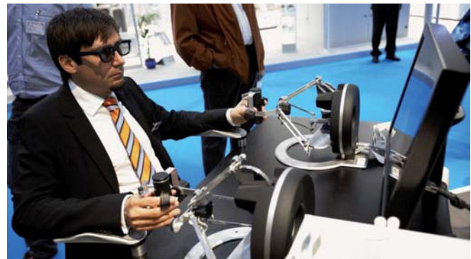
Fig. 5. Surgeon's workstation with two haptic devices and a stereo display with polarized light
