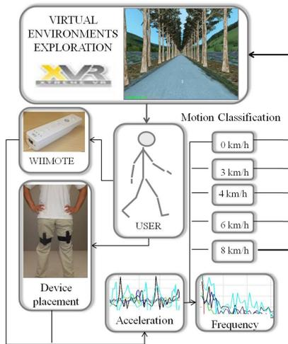
Fig. 2. Block diagram of the speed locomotion recognition.
