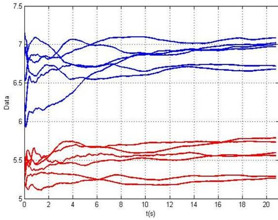
Fig. 8. Rate recognition of 6 different samples of 5.5km/h (red line) and 7km/h (blue line) velocities during 21 seconds test.
