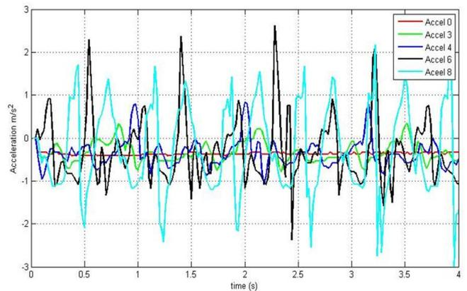
Fig. 4. Acceleration data obtained at 4 min from the velocities of: 0km/h, 3km/h, 4km/h, 6km/h and 8km/h.
