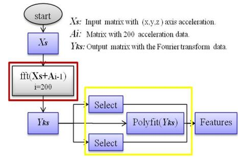
Fig. 9. Feature extraction process, the red block represents the recursive process to estimate the FFT (cf. fig. 10, the state machine block), while the yellow block represent the feature extraction process (cf. fig. 10, the feature extraction block).
