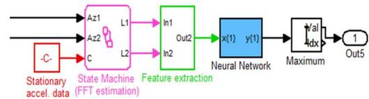
Fig. 10. Simulink implementation of the phase classifier.
