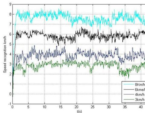
Fig. 13. Signals of the speed recognition online, obtained by the user's locomotion using a treadmill during 42sec.
