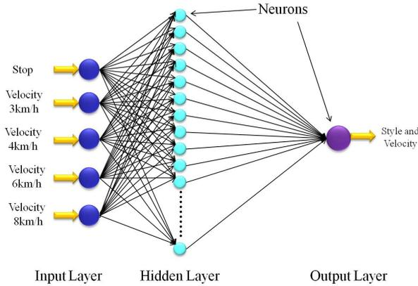
Fig. 6. A feed-forward multilayer perceptron (MLP) network with 20 neurons.
