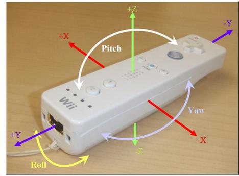
Fig. 3. Wiimote controller device with the axes reference.
