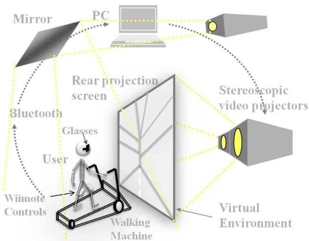
Fig. 11. The full system setup (the use of the treadmill for the interaction is optional).
