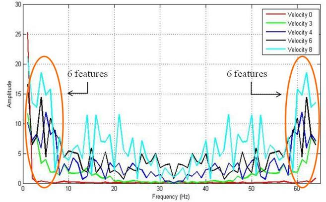
Fig. 5. Windows of the absolute value of the Fourier transform for each 200 acceleration samples.
