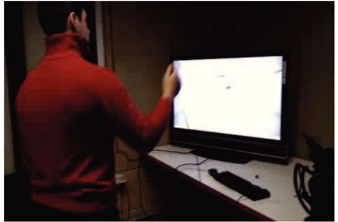
Fig. 5. The system used during the experiment. The user stands in front of a monitor where a virtual hand and a virtual ball are shown. The user controls the position of the virtual hand moving a Polhemus® tracker.
