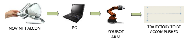
Figure 4. Unilateral teleoperation workflow: the three degrees of freedom of the robotic arm are mapped to the haptic device position. A moving reference strategy is implemented to allow the user to move the robotic-arm only when he pushes a button on the handle. The orientation can be changed only between moving phases using a second button on the handle.
