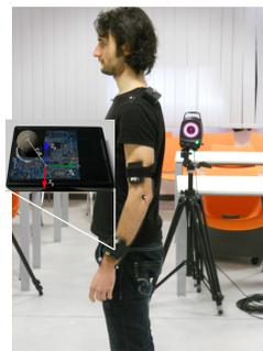
Fig. 3. Experimental setup for synchronized IMUs and optical motion capture. Sensor frame with offset  $r_{off}$  from actual sensor frame origin and marker center in the magnified area.
