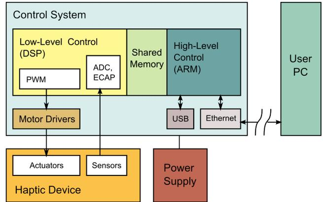
Fig. 2: Overview of the system modules and connections. Relevant control parameters are shared between the DSP and the ARM-CPU cores controller using a shared memory mechanism. The ARM controller implements a web server and provides to generate a local haptic response loop which reacts to networked commands.
