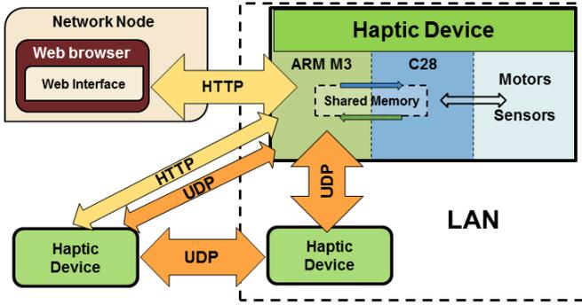
Fig. 5: Overall system and communication architecture. The haptic interface is described in terms of its connection with other haptic devices or with external computing nodes. The main communication channel with other devices is UDP, supported by HTTP for handshaking and communication.
