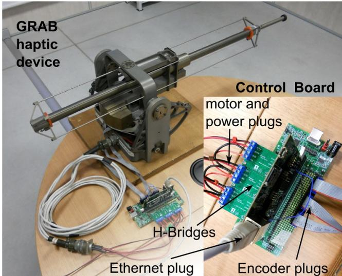
Fig. 1: Overview of the GRAB [13] haptic interface integrated with the proposed electronic controller.
