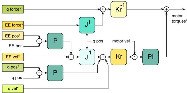
Fig. 3: Low-level control architecture
