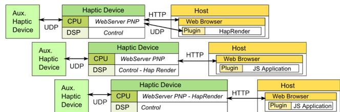
Fig. 4: Different possibilities for the haptic rendering configuration with the proposed architecture. Remote web-client rendering (top); DSP low level rendering (middle); and ARM-CPU Rendering (bottom).
