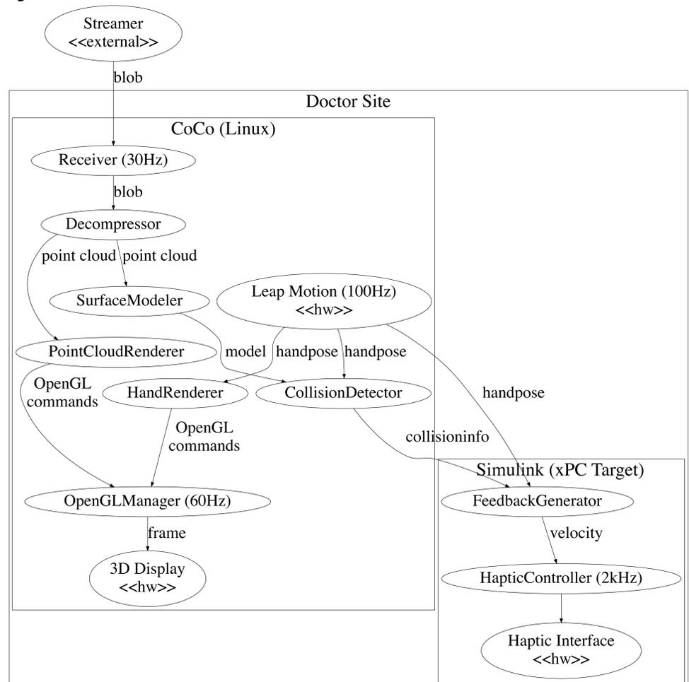
**A new framework for high-performance AR/VR Compact Components (CoCo):** core library + AR + application components.
