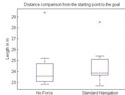
Fig. 7: Standard Navigation: distance traveled.
