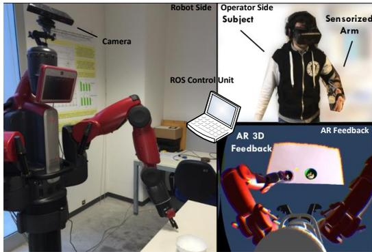
**Figure 1:** The system architecture. Synchronized raw sensors data are captured and sent via Bluetooth to the host PC by the wearable device. Gathered data are used to extract motion and muscle efforts information. The computed data are used by a ROS control node to operate a robot arm. An augmented visual feedback of the scenario with which the robot is interacting is provided to the user.
