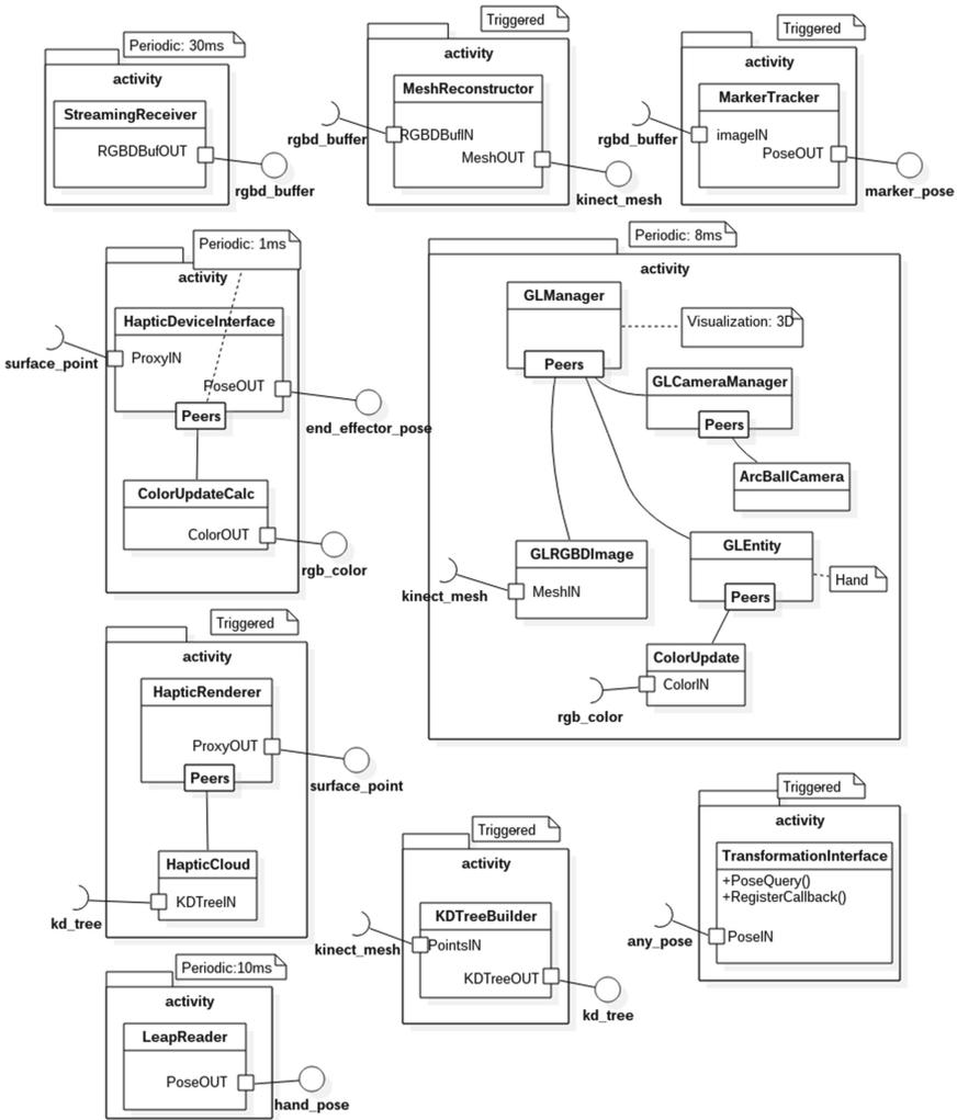
**Fig. 4.** CoCoMR components involved in the visuo-haptic application. Port with the same name type are connected to each other. Every poses pass through *TransformationInterface* to be transformed in the correct reference system.
