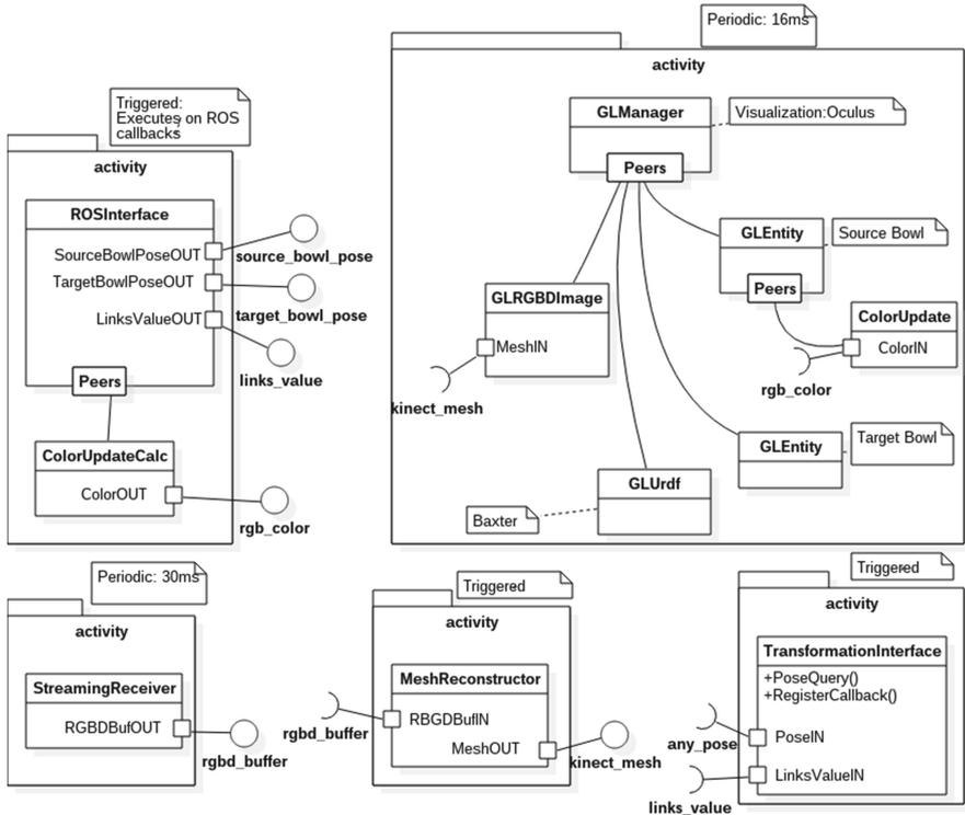
**Fig. 6.** CoCoMR components involved in the teleoperation application. Port with the same name type are connected to each other. Every pose passes through *TransformationInterface* to be transformed in the correct reference system.
