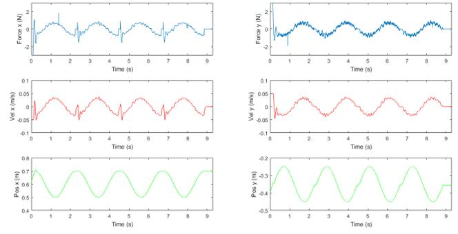
Fig. 6. Comparison between force exerted, velocity commanded and actual position while performing circular trajectory.
