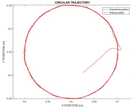
Fig. 4. Trajectory tracking performed by Motore++ system. The maximum error is 0.0029 m, calculated as the difference between the maximum radius obtained and the desired radius.
