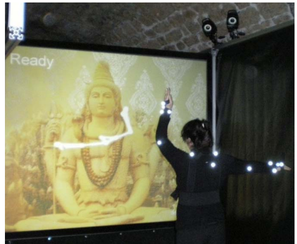
Fig. 4. The recognition system in action. It is possible observe how the cameras track the user movements using the reflective markers that are mounted on the suit dressed by the user. The user's avatar and the image that represents the meaning (a King) of the recognized gesture are displayed in the screen.
