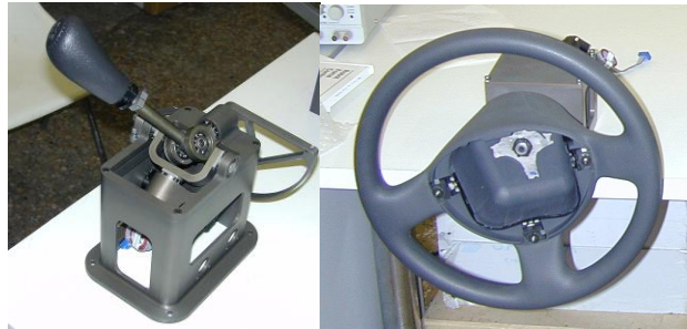
Figure 3 Specialized haptic device for providing force feedback in driving simulator. These systems provide a flexible and realistic force feedback. Compare them with the general haptic interface used in Fig. 1 left.
