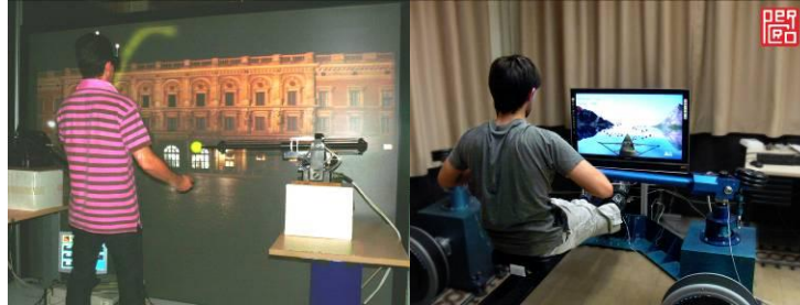
Figure 6 Two examples of systems for training based on the multimodal training schema. On the left the Haptic Juggling with co-located feedback, and on the right the Rowing System providing realistic water feedback.
