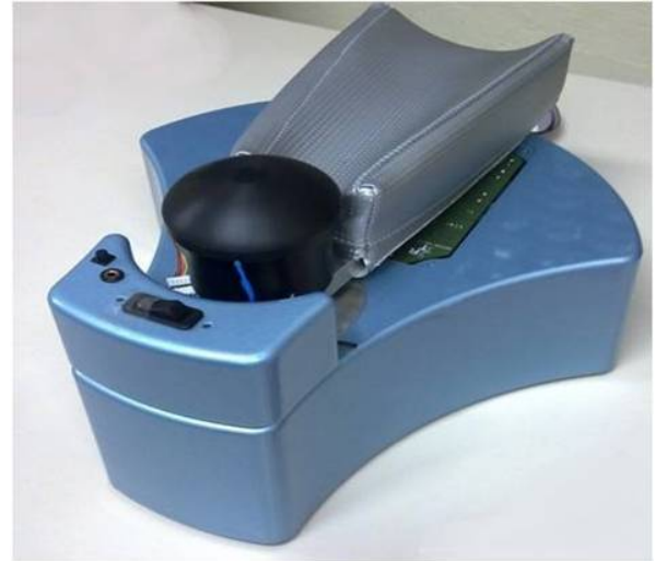
Figure 1: MOTORE: Portable Haptic Interface. The photo shows the device with main body in blue, the handle in black, that is grasped by the user and the forearm support in grey.
