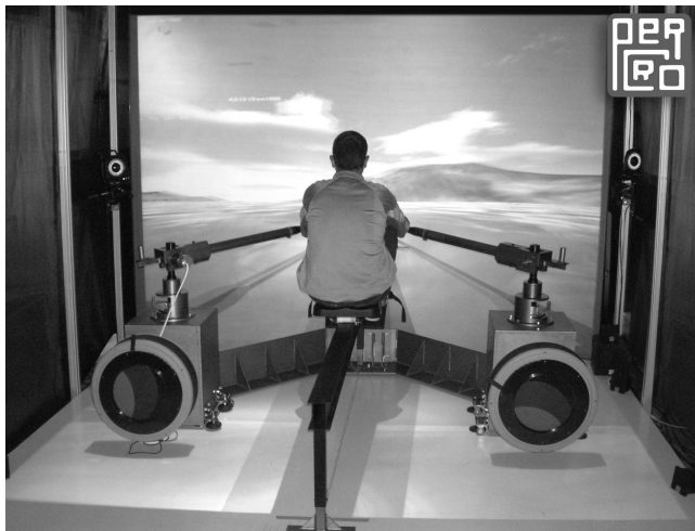
Figure 2. SPRINT system configured inside an immersive visualization system.
