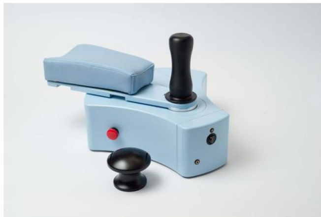
Fig. 1: MOTORE: MOBILE roboT for upper limb neuroREhabilitation. The picture shows the rehabilitation tool with the two handles designed for different kind of patients.
