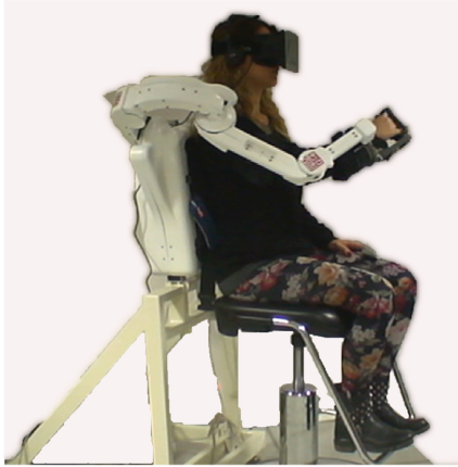
(a) Immersive setup used for the experiment. The subject is seated wearing the Oculus HMD and the ALEX exoskeleton
