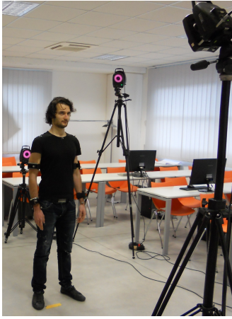
Fig. 5. Experimental setup with the IMUs mounted on the participants limb as well as the Vicon system markers.
