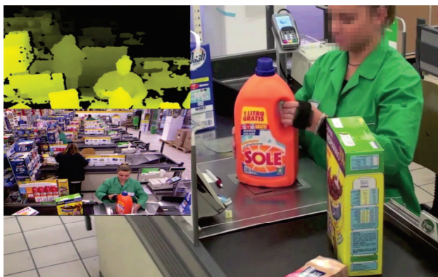
Fig. 5. Three views of the setup in the preliminary test. On the right the main scene captured with a camera. On the left the views of the RGB-D sensors that allow to understand the organization of the workspace. The RGB-D could be used for improving the tracking of body motions and interaction with the objects.
