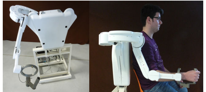
Fig. 1. ALEx exoskeleton and a user wearing it.
