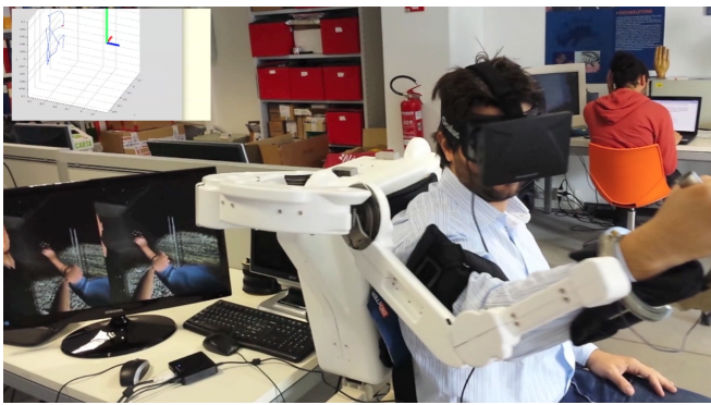
Fig. 2. User moving its own virtual arm using the ALEX exoskeleton and the Oculus Rift.
