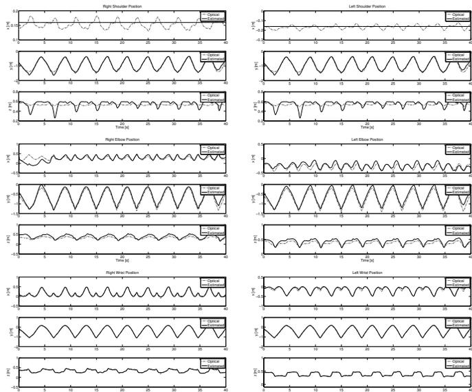
Fig. 3. Motion tracking results obtained with the inertial tracking system algorithm for the first rowing trial (Shoulder, Elbow and Wrist positions).
