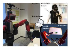
**Figure 1:** The system architecture. Synchronized raw sensors data are captured and sent via Bluetooth to the host PC by the wearable device. Gathered data are used to extract motion and muscle efforts information. The computed data are used by a ROS control node to operate a robot arm. An augmented visual feedback of the scenario with which the robot is interacting is provided to the user.
