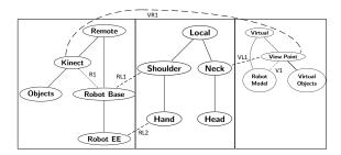
**Figure 3:** The transformation graph describing the connection between the relevant reference frames. Local frames are related to the user side, while Remote frames comprises all the reference frames from the remote manipulator side. Virtual frames are the ones represented in the 3D virtual environment. Fixed transformations between the frames (dashed lines) are computed with the calibration procedures.
