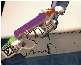
**Fig. 2.** Result of the registration of the Kinect with the robot kinematics. The image part is a rendering of the Kinect point cloud, while the colored parts are meshes from the URDF controlled by robot joints. Finally in the lower left the calibration fiducial marker is visible.
