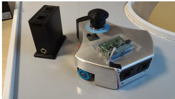
Fig. 1. MOTORE++: The new version of the Portable Haptic Interface. Battery charger with replacement battery (left). The device, with the radio unit and programming board (right). The sliding panel with textured pattern (bottom).
