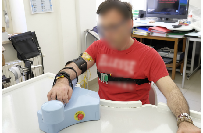
Fig. 1. User interacting with the MOTORE++ device: the user sits at the desk holding the device handle where a XY force cell is present. The arm is resting on the arm holder. A counterweight is used to balance the device. During rehabilitation exercises, the user can move the mobile robot all over the desk. In the meanwhile the user wears the wearable 5 DoF system. The armband on the upper arm contains an IMU unit and the EMG add-on, while the other two bands at wrist and torso contain IMU units.
