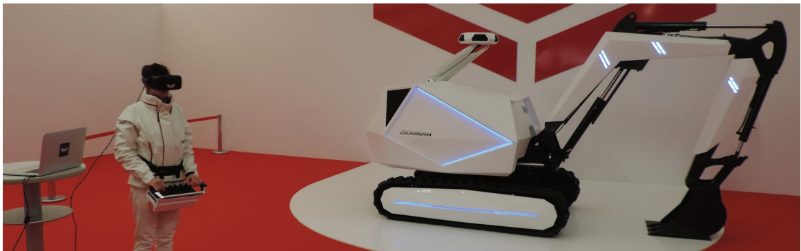
Figure 2. Final system with the operator on the left and the working machine on the right. The vision head can be seen on top of the machine.
